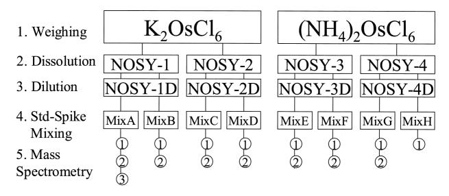
Fig. 1. Flow chart for preparation of Os gravimetric standards (NOSY-1, NOSY-2, NOSY-3, and NOSY-4) from  $K_2OsCl_6$ and  $(NH_4)_2OsCl_6$ , dilution of these standards, and preparation of the eight mixtures (MixA through MixH) of diluted standards with Os spike (HOST1). The isotopic composition of Os was measured by MC-ICP-MS at least twice for each mixture (except MixH).
