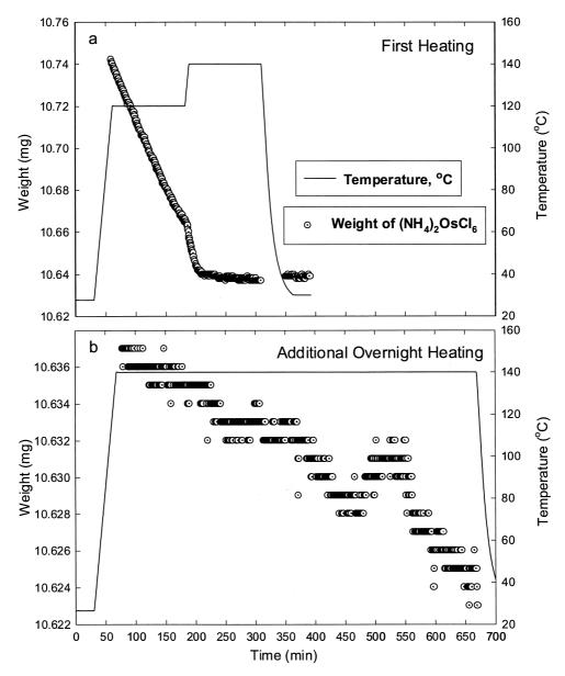
Fig. 3. Thermal gravimetric analysis results for  $(NH_4)_2OsCl_6$ . (a) shows rapid weight loss of  $\sim 1.0 \pm 0.1\%$  within first few hours. This is interpreted to reflect evaporation of absorbed water. After  $\sim 3$  hours, the rate of change is much less. (b) Further heating results in continuous weight loss at a much slower rate. Each data point represents the weight recorded every 30 seconds.
