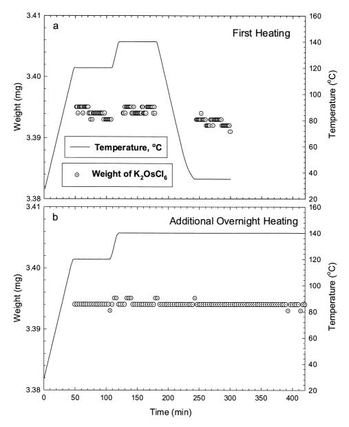
Fig. 2. Thermal Gravimetric Analysis results for  $K_2OsCl_6$ . (a) shows first 300 min of heating and (b) an additional 420 min. The lines represent the heating pattern (temperature in °C). The open circle data points record weight changes in  $K_2OsCl_6$  in mg, measured every 3 min. The temperature range for heating (120–140°C) was selected based on the recommendation of Gilchrist (1932) and adopted by Morgan et al. (1995) and Birck and Allègre (1998).
