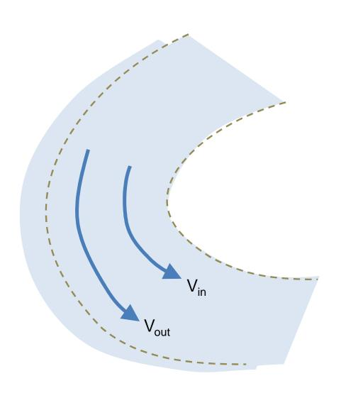
$$V_{out} = \frac{R_{out}}{R_{in}} V_{ir}$$
